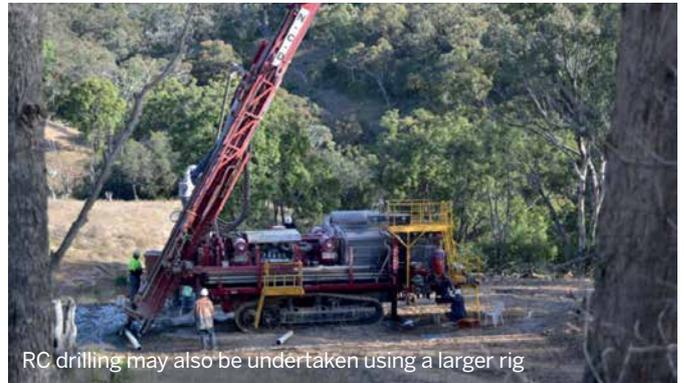
RC drilling may also be undertaken using a larger rig
