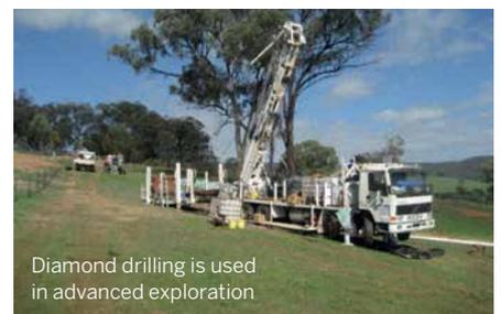
Diamond drilling is used in advanced exploration
