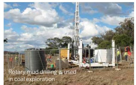
Rotary mud drilling is used in coal exploration
