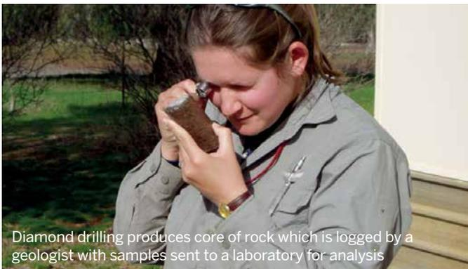
Diamond drilling produces core of rock which is logged by a geologist with samples sent to a laboratory for analysis
