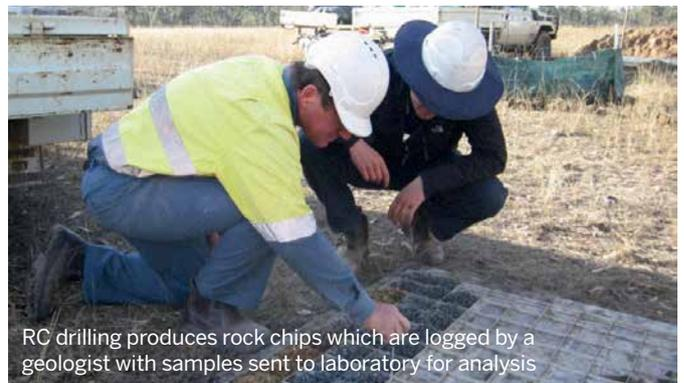
RC drilling produces rock chips which are logged by a geologist with samples sent to laboratory for analysis
