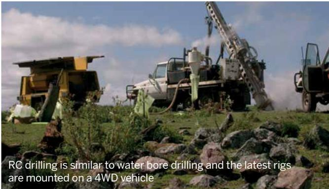
RC drilling is similar to water bore drilling and the latest rigs are mounted on a 4WD vehicle
